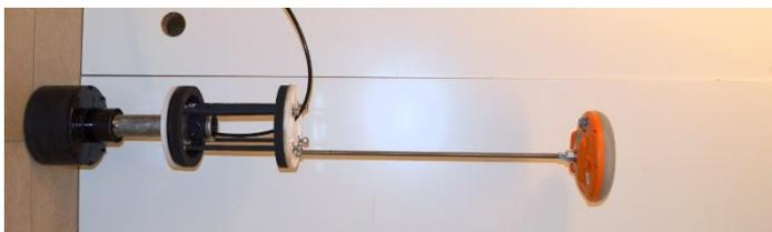
Put the cable through the bracket, then screw the hydrobook onto the bracket.
