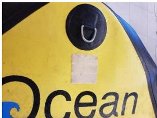
On the bow of the calypso inflatable boat, a Velcro patch is provided to place the compass and keep it in place.
