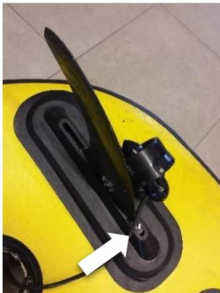
Turn the vessel around. To place the motor fins correctly, make sure that the motors are on the outside. Slide the fins in their place and fasten the bolt to secure that the motor no longer comes loose. Put the two cables of the motors through the closest hole of the vessel and turn the boat around again.
